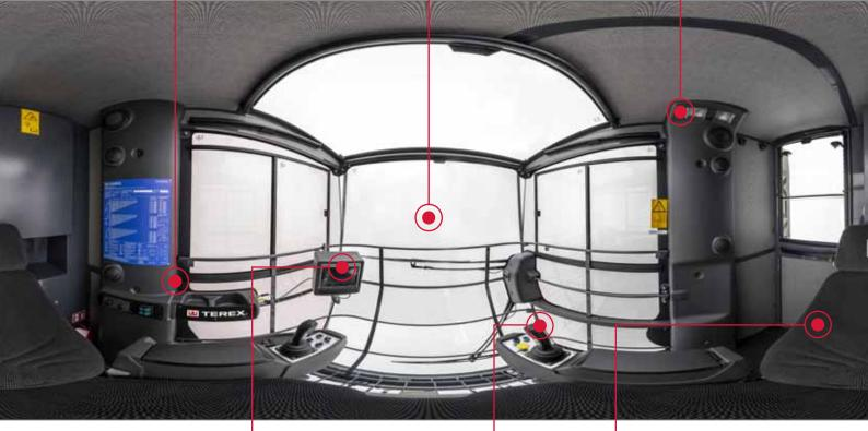
Display & control system: expanded configuration options to meet different jobsite needs. Quick set-up, Terex Power Plus, Power match and auto-leveling are functions to enhance your daily work.
